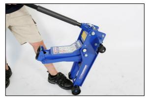
6. Ensure lift arm returns to fully lowered position
