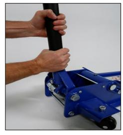
3. Pump With the help of an assistant stand the jack on its end on the edge of a bench.
