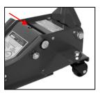
7. All lower lift arm pivots and pins in all linkages should be cleaned using an aerosol degreaser and after drying should be lubricated with a Light Bearing Grease or 30/40W Machine Oil to ensure long life and prevent premature wear.
