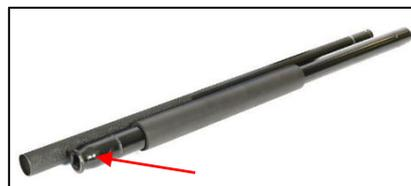
4. The handle socket pivots and bolts should be cleaned using an aerosol degreaser and after drying should be lubricated with 30w/40w oil to prevent premature wear of the handle socket pivot bolts.
