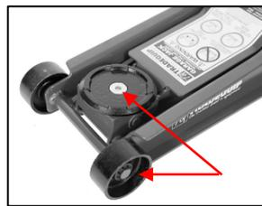
2. Wheels Castor axles and bearing races should be cleaned using an aerosol degreaser and after drying lubricated with a Light Bearing Grease or 30/40W Machine Oil to ensure long life and prevent premature wear and provide smooth rotation during positioning and lifting.
