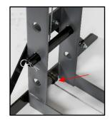
4. Periodically extend, clean, and lubricate the ram shaft with silicone lubricant spray to ensure smooth extension and retraction of the ram. Where applicable clean and lubricate the threaded adjustor with Light Bearing Grease or 30/40W Machine Oil.
