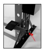
2. Bed load bearing surfaces should be lubricated with a Light Bearing Grease or 30/40W Machine Oil to ensure long life and prevent premature wear.
