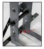
4. Periodically extend, clean, and lubricate the ram shaft with silicone lubricant spray to ensure smooth extension and retraction of the ram.
