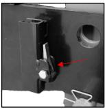
7. Lubricate Winch mechanicals including Gears, Axle Rods and Ratchet Assemblies.
