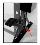
2. Bed load bearing surfaces should be lubricated with a Light Bearing Grease or 30/40W Machine Oil to ensure long life and prevent premature wear.
