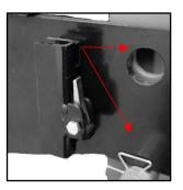
6. Lubricate the safety guard latches periodically to ensure easy guard height readjustment.
