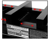
3. Bed winch pulleys should be lubricated with a Light Bearing Grease or 30/40W Machine Oil to ensure smooth operation, long life and prevent premature wear.
