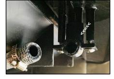
4. Remove the broken barb end of the elbow from the water supply hose.
