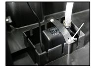
8. Reattach the cable to the loom with new cable ties and rewind the insulation up to the lower bulkhead.
