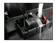
5. Remove the 6 Control panel screws and reveal and unplug the Pump Cable from the rear of the circuit board.
