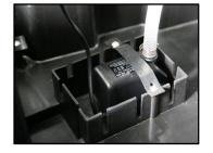
4. Remove the pump retainer and lift the pump [item 28] from the base of the water tank.
