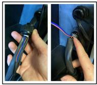
10. Connect the pump cable plug to the control panel then loop the extra cable and cable tie it, tucking this behind the control panel. Refit the control panel with the screws. Ensure the thread cable and cable braid back together.
