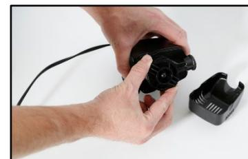
7. Pull the impeller from the main pump housing.
