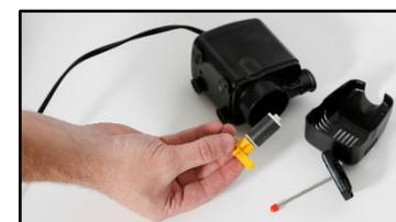
8. Install new impeller.
