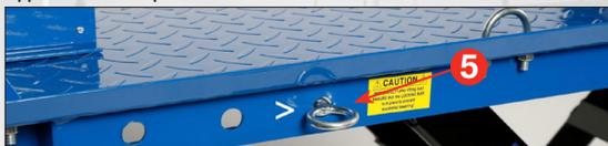
Raise to the desired height then insert the pin and operate the hydraulic release to take load onto the locking device assembly.
