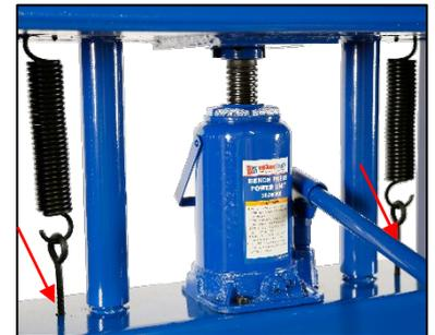
2. Remove the Bottle Jack base mount screws and gently remove the jack from the frame and place on a suitable work bench for the bleeding procedure to continue.
