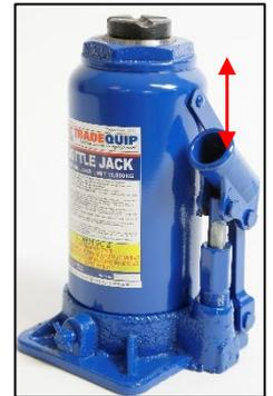
7. Invert the jack and push the pump socket assembly back to the horizontal position.
