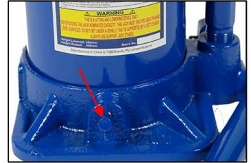
6. With the jack on its base pull the pump socket upwards to the raised position.
