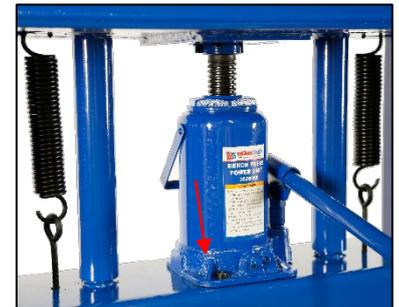
3. Remove the Filler Bung and if required, refill with \*32 Grade Hydraulic until the oil is lapping the bottom of the filler hole then replace the Filler Bung.
