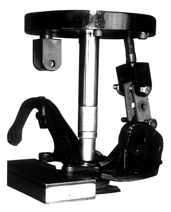
Removal and assembly of bearings. Common tool.
