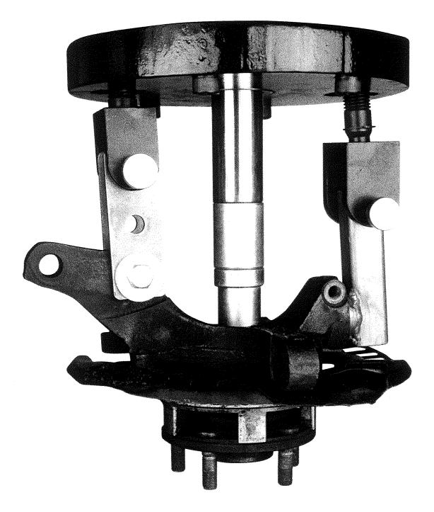
Hub replacement to bearing assembly using tool's supplied.
