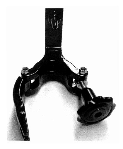
Standard way of holding common Japanese hubs. Note adjustment screws.
