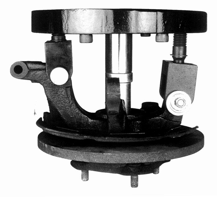
Holding larger size hubs using hanging brackets supplied
