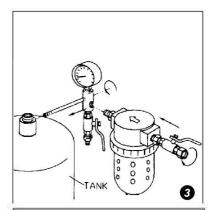
3. Step 4, assembly of the sand outlet valve into the opening at the bottom of the tank. Attach in order; nipple connector (17), sand metering valve (19B), nipple connector (17), and sand outlet pipe (25).
