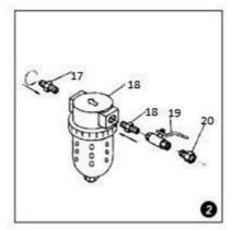
3. Step 3, place the tank (01) on a table with the four clips up. Screw the water trap filter (18) and its parts into the opening at the side of the intake manifold. Then screw the open end of the joint pipe (14) with intake manifold (15) and pressure gauge (17) attached into the threaded opening on the side of the filler pipe on top of the tank. Be sure that the manifold and gauge are vertical.
