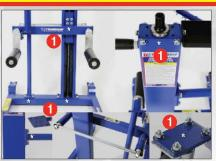
Safe operation of your Wheel Tyre Lifter. To ensure safe operation of your Wheel Tyre Lifter whilst under load, always make sure the roller legs are at 90 degrees to the vehicle wheel and the wheel safety clamp is correctly positioned to allow for smooth operation while raising, lowering, and relocating the wheel.
