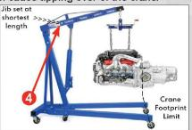
Use the jib settings to create a balanced load within the footprint of the crane.
