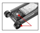
2. Wheels Castor axles and bearing races should be cleaned using an aerosol degreaser and after drying lubricated with a Light Bearing Grease or 30/40W Machine Oil to ensure long life and prevent premature wear and provide smooth rotation during positioning and lifting.
