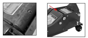
7. All lower lift arm pivots and pins in all linkages should be cleaned using an aerosol degreaser and after drying should be lubricated with a Light Bearing Grease or 30/40W Machine Oil to ensure long life and prevent premature wear.
