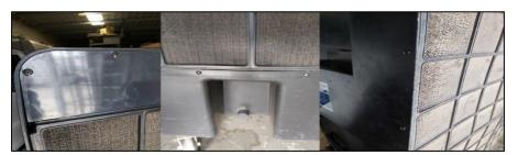
3. Remove the cooling pad and set aside.
