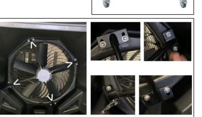
Remove the rear mesh protection screen and cooling pad and set aside
