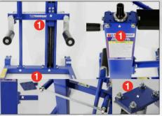
2 Regularly lubricate all castors and wheels for ease of movement once loaded.
