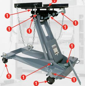
Always store in the fully lowered position. Storage in the lowered position ensures the lift ram assembly is sealed from exposure to weather fluctuations and keeps the hydraulic ram seals in a relaxed condition ready to work when required.
