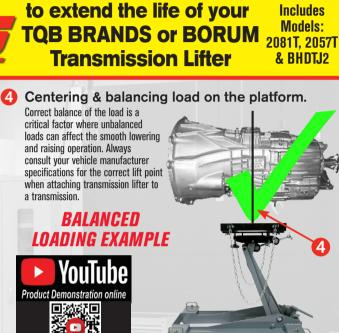
Use correct model for intended applications. The following chart explains model suitability based on GVM and Transmission type.
