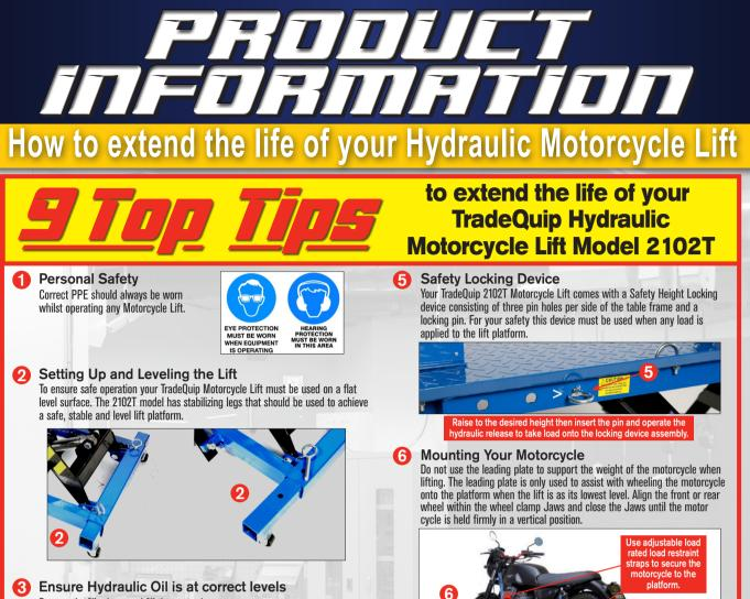
Remove the filler bung and fill the reservoir with SAE 32 hydraulic oil to within 5mm to 10 mm below the filler hole. Replace the filler bung and test the jack throughout its entire stroke to ensure full stroke is achieved adding additional oil as required.
