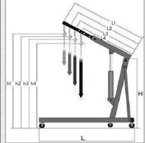
4 Off centre loading and unbalanced loads or loads that mount outside of the crane's footprint can cause tipping over of the crane.
