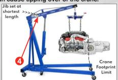
5 Use the jib settings to create a balanced load within the footprint of the crane.
