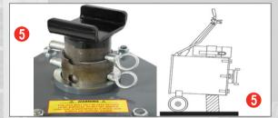
6 Off centre loading or unbalanced loads can affect the smooth lowering and raising operation. Always consult your vehicle manufacturer specifications for the correct lift point. Never lift from a suspension pivot or air bag mount plate where these items are designed to travel in an arc causing excess lateral force to the jack throughout its lift cycle.
