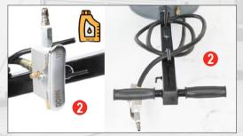
A periodic coating of light lubricating oil such as 30/40W Machine Oil to all lift ram shafts of the jack will help to prevent rust and assure that they move freely.
