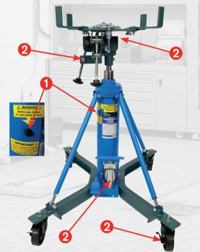
3 Always store in the fully lowered position. Storage in the lowered position ensures the lift ram assembly is sealed from exposure to weather fluctuations and keeps the hydraulic ram seals in a relaxed condition ready to work when required.
