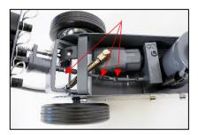
7. Regularly wind the screw extension to full length, clean with a suitable degreaser and apply a light bearing grease to ensure smooth operation when in use.
