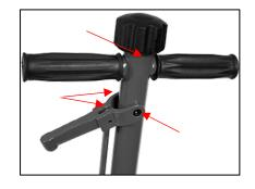
5. Lubricate the release mechanism spigot and handle position locking Pin with 30w/40w oil to prevent premature wear of the release drive and locking pin.
