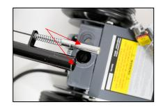
6. Remove the top cover and lubricate the release universal joint with a light weight bearing grease to ensure smooth operation. Replace the top cover after lubrication.
