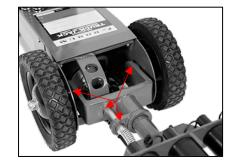
4. Lubricate with a Light Bearing grease the release knob and locking pin handle assembly with 30w/40w oil.
