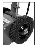
3. Lubricate handle socket pivots and positioning locking pin with a Light Bearing Grease to provide smooth operation from vertical to horizontal positions.
