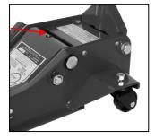
9. All lower lift arm pivots and pins in all linkages should be lubricated with a Light Bearing Grease or 30/40W Machine Oil to ensure long life and prevent premature wear.
