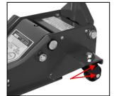
3. Lubricate handle socket with a Light Bearing Grease to provide smooth operation from raise to release position.
