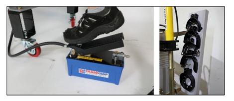
9. Recheck the oil volume in the pump as per step 2 and top up as necessary.
