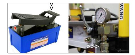
2. With pump in its upright, horizontal position, remove the oil filler plug located on the top plate of the reservoir. Use a small funnel to fill reservoir to within 19mm of the opening. Wipe up any spilled fluid and reinstall the oil filler plug.
