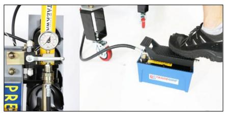
7. Turn the switching tap to "spring compressor" and depress the pump pedal and extend the spring compressor ram to approximately 50% of travel. Hold in this position for 20 seconds to allow air to settle.
