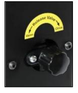
4. Close the release valve and insert the pump handle into the socket of manual pump and pump the handle until the ram is at full stroke, then open the release and allow the ram to fully retract.
