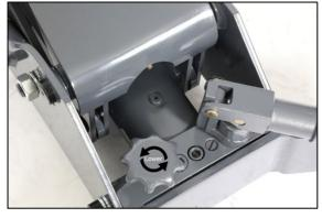
3. With one foot on the front castor mount assembly, slowly raise the lift arm by hand to three quarter height and release, the lift arm will slowly fall back to lowered position. Repeat this process 3 to 4 times.
