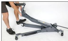
4. Remove the oil filler bung from the hydraulic ram to release any air pressure or vacuum buildup. If required, refill with \*32 Grade Hydraulic until the oil is approximately 6mm below the filler hole.
