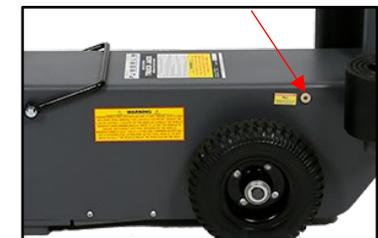
At this point the Air Motor Pump and Lift Ram should be free of air and the Jack ready for operation. If the jack continues to show the symptoms as above repeat the steps 1 to 5 or please refer to a Qualified Hydraulic Technician.
