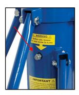
2. To successfully bleed the Transmission Lifter, we begin with the pump, start by depressing the release pedal and hold it in the release position while pumping the pump pedal 10times. Once the pump regains firm resistance throughout its stroke and upwards movement is seen at the lift rams, move on to Step 3.
