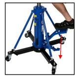
4. With an Allen key undo the Lift Ram bleed screw 1 full turn anticlockwise, aerated oil will begin to exit the bleed screw housing until a clear stream of oil with no air bubbles flows. Tighten the pump bleed screw and raise the pedal to fully raised position.
