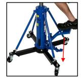
3. Pump the lift rams to full extension. With an Allen key undo the Lift Ram bleed screw 1 full turn anticlockwise. Aerated oil will begin to exit the bleed screw housing until a clear stream of oil with no air bubbles flows. Tighten the pump bleed screw and test for rebound by applying downwards pressure against the upper lift ram.
