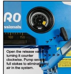
**Air Pump:** open the release valve by turning it counter clockwise. Connect the quick coupler-male into the air supply hose quick coupler-female, then turn on the air valve letting the pump work for several times to eliminate any air in the system.
