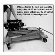
Remove the oil filler bung from the top of the hydraulic ram and turn the release valve anticlockwise to open.
