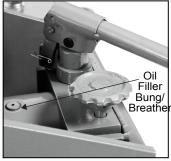
2. Leaving the Pump Handle in the lowered position, open the release knob one eighth turn anticlockwise.
