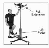
4. While holding the pedal down open the release handle till the pedal starts to slowly drop keeping a firm resistance feel in the pedal. Continue to pump the pump pedal approximately 10 times then open the release and allow the lift ram to completely retract.
