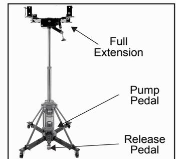
5. With the Release Pedal wedged open, begin to pump the Pump Pedal approximately 10 times then remove the wedge from the Release Pedal
